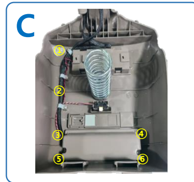
C. After removing the screws in the numbered order, open main board cover
