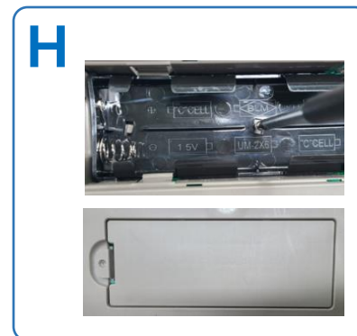
H. To fix the battery holder to the body frame, insert a screw into the center of battery holder
